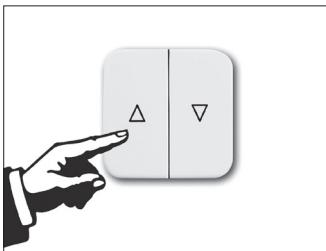
Move the awning with the ▲ (Up button) into the front rail stop until the motor switches off automatically.
