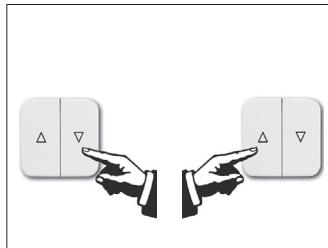
Extend the awning with the ▼ (DOWN button) until the front rail stop can be operated.
